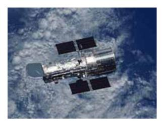
The Hubble Space Telescope uses photocells to generate the electricity it needs — image courtesy of NASA.
